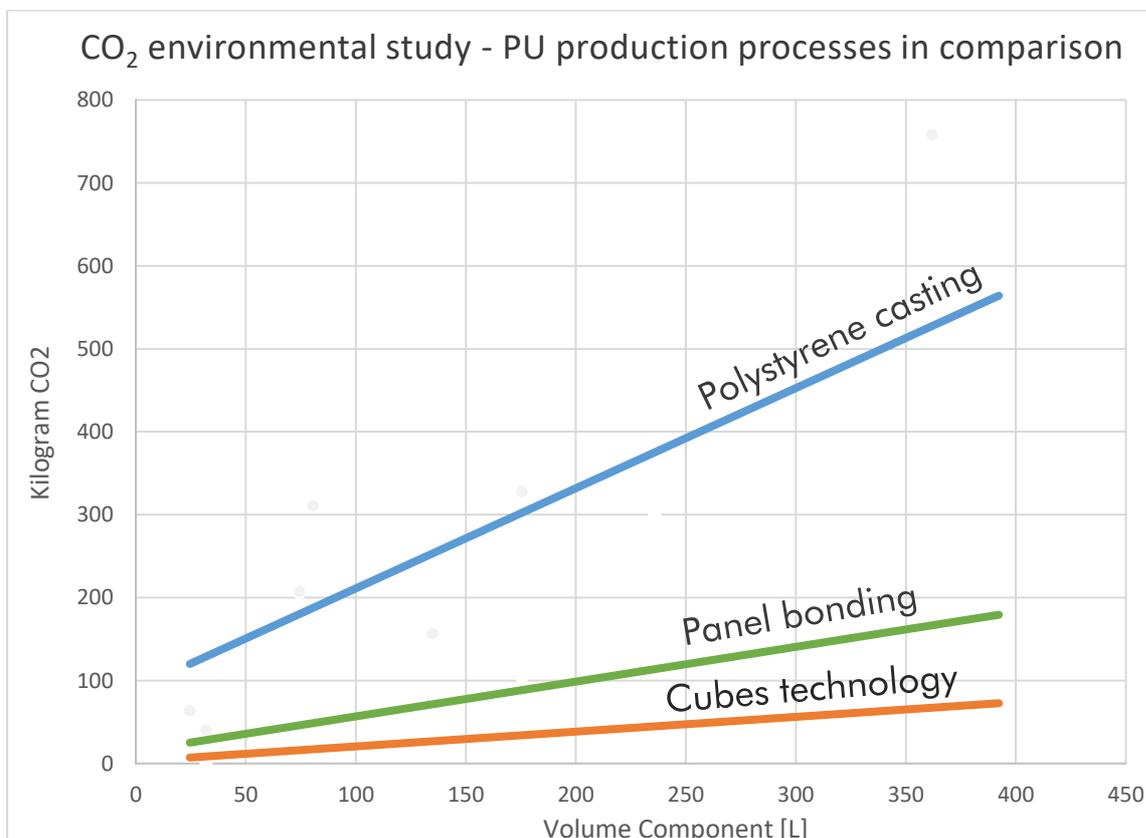
Due to the large influence of the geometries, there is a wide scatter in polystyrene casting. However, the slope of the regression line still provides a very good approximation for estimating the CO<sub>2</sub> emissions of future projects
